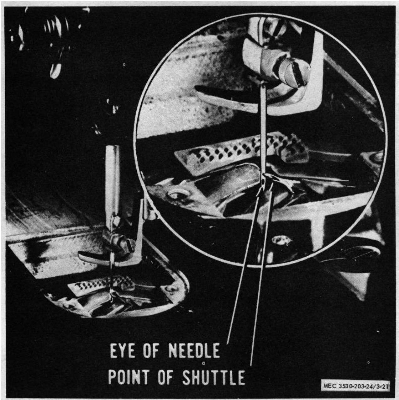
Figure 3-21. Correctly timed needle on clothing sewing machine.
